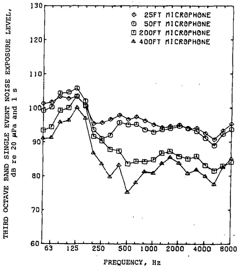
Figure 14a. Single event noise exposure level versus frequency for train no. 3555.
