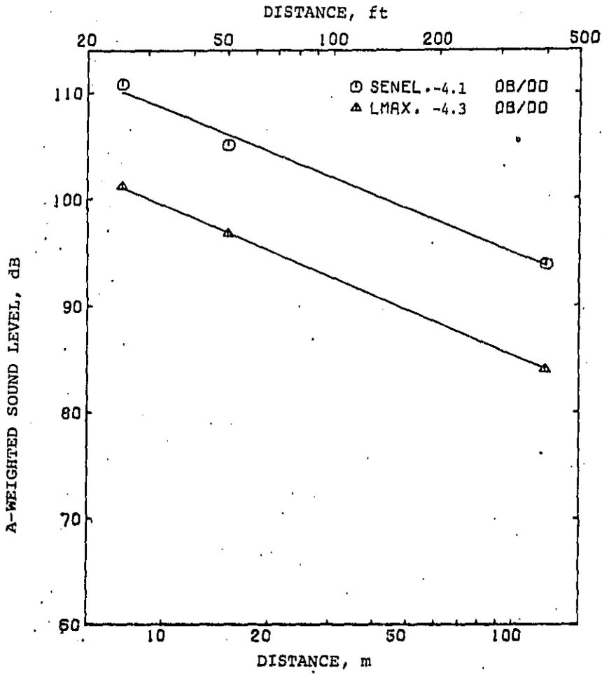
Figure 13b. Maximum A-weighted sound level (in dB re 20  $\mu$ Pa) and A-weighted SENEL (in dB re 20  $\mu$ Pa and 1 second) versus distance for train no. 4031.
