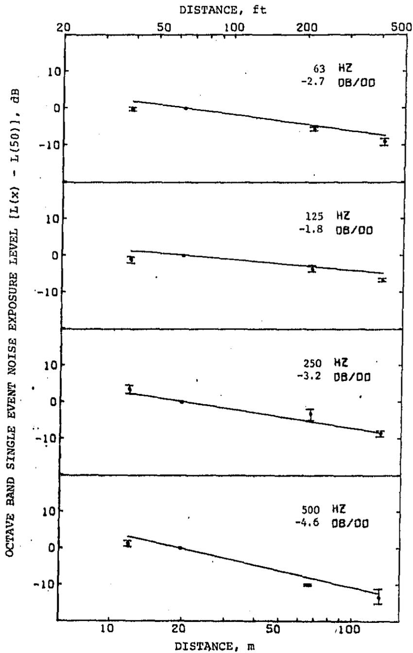
Figure 16a. Octave band SENEL [L(x) - L(50)] versus distance for east bound trains.
