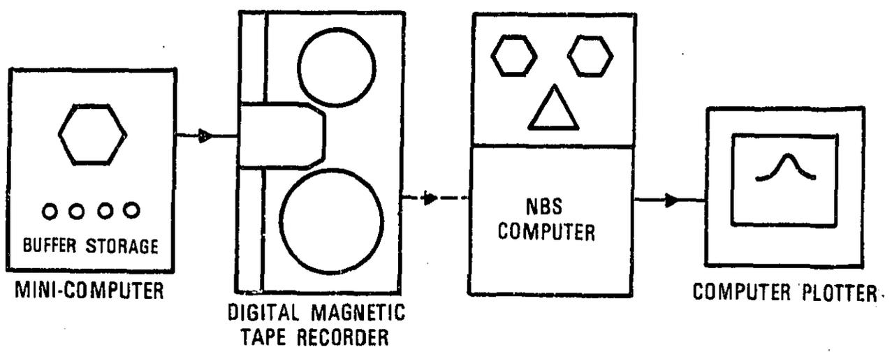
Figure C-2. Data reduction and analysis system for yard noise.
