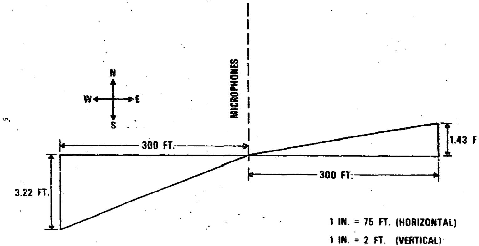
Figure 3. Track elevation 300 feet on either side of the intersection point of the track and the line of microphones.
