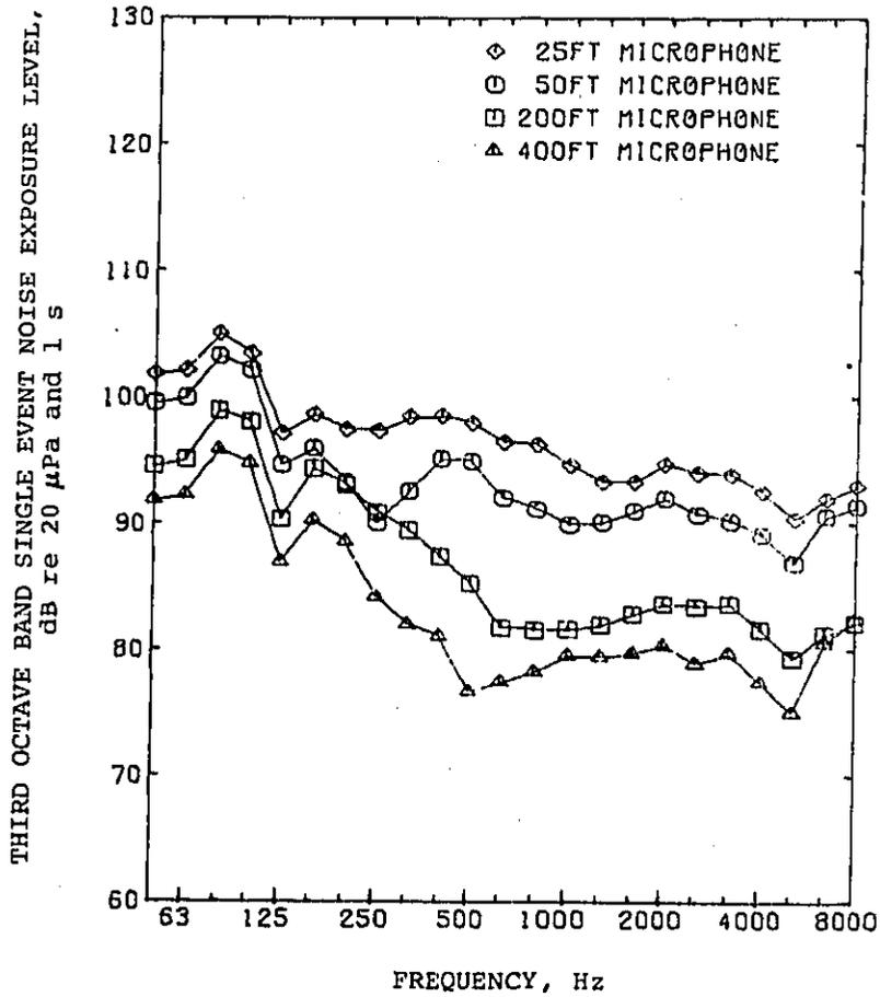
Figure 11a. Single event noise exposure level versus frequency for train no. 4548.
