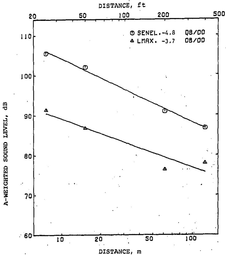
Figure 7b. Maximum A-weighted sound level (in dB re 20  $\mu$ Pa) and A-weighted SENEL (in dB re 20  $\mu$ Pa and 1 second) versus distance for train no. 7411.
