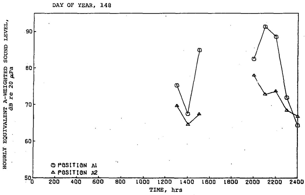
Figure 32b. Hourly equivalent A-weighted sound level versus time.
