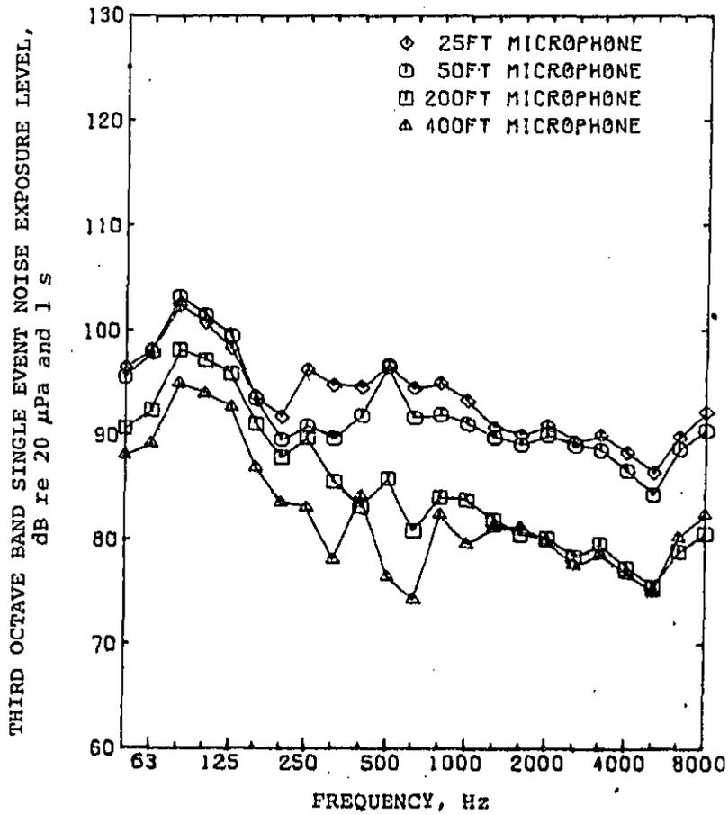
Figure 15a. Single event noise exposure level versus frequency for train no. 6955.
