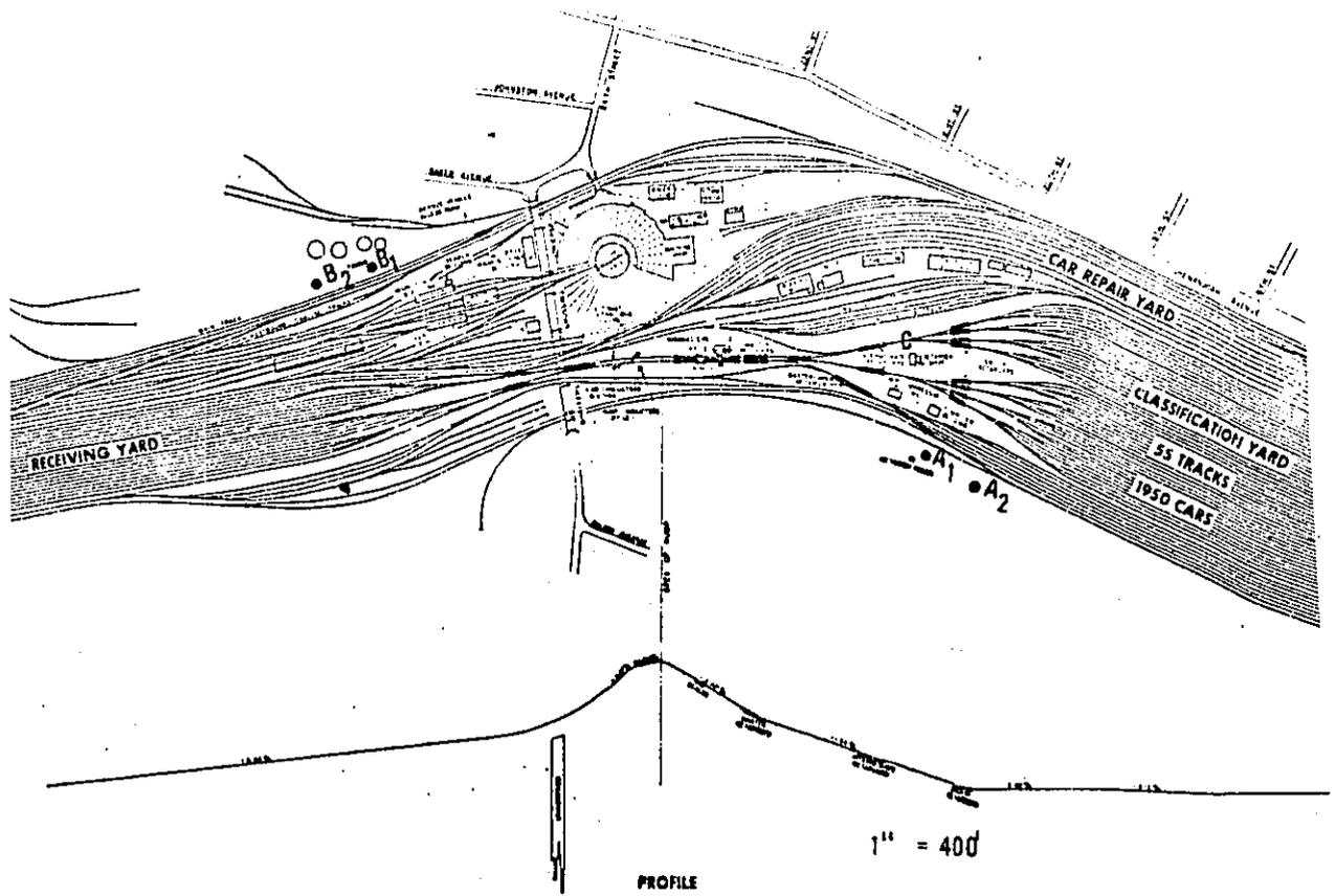
Figure 23. Layout of the Norfolk and Western Railroad Terminal, Roanoke, Virginia, showing microphone locations, designated A1, A2, B1, B2, and C, for rail yard noise measurements.
