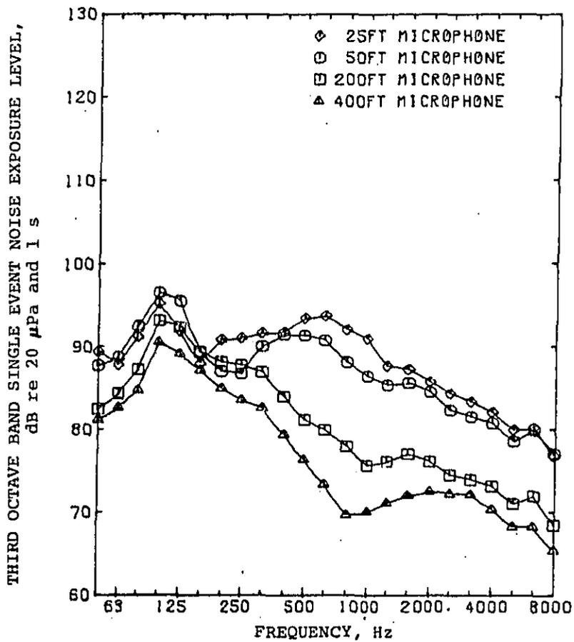
Figure 6a. Single event noise exposure level versus frequency for train no. 6607.
