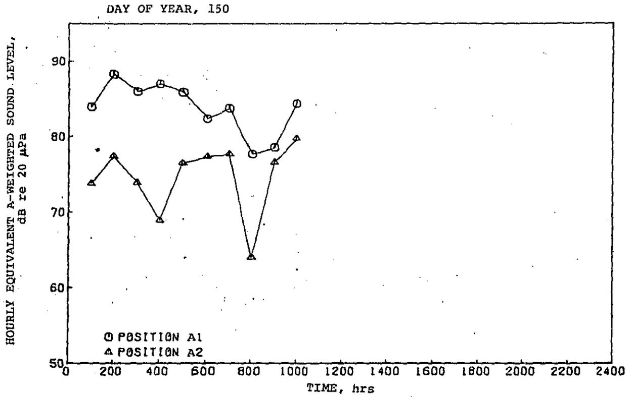
Figure 34b. Hourly equivalent A-weighted sound level versus time.
