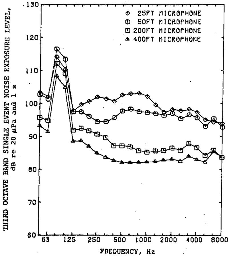
Figure 10a. Single event noise exposure level versus frequency for train no. 4036.
