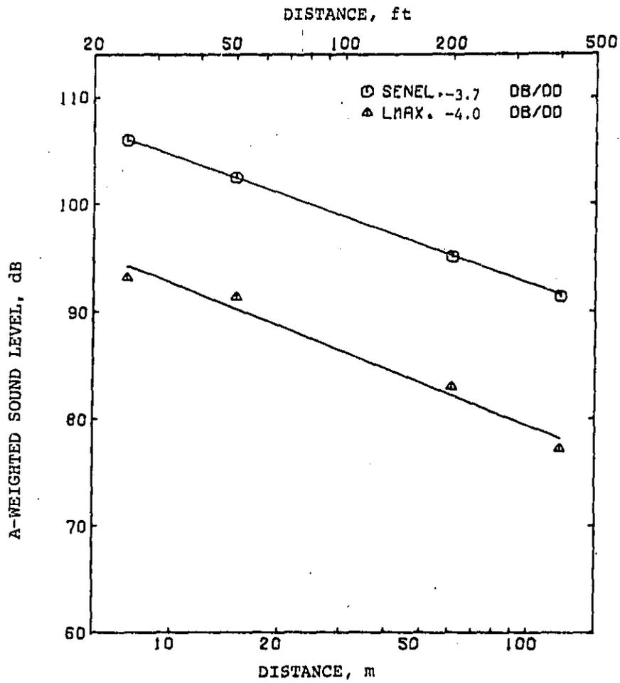
Figure 11b. Maximum A-weighted sound level (in dB re 20  $\mu$ Pa) and A-weighted SENEL (in dB re 20  $\mu$ Pa and 1 second) versus distance for train no. 4548.
