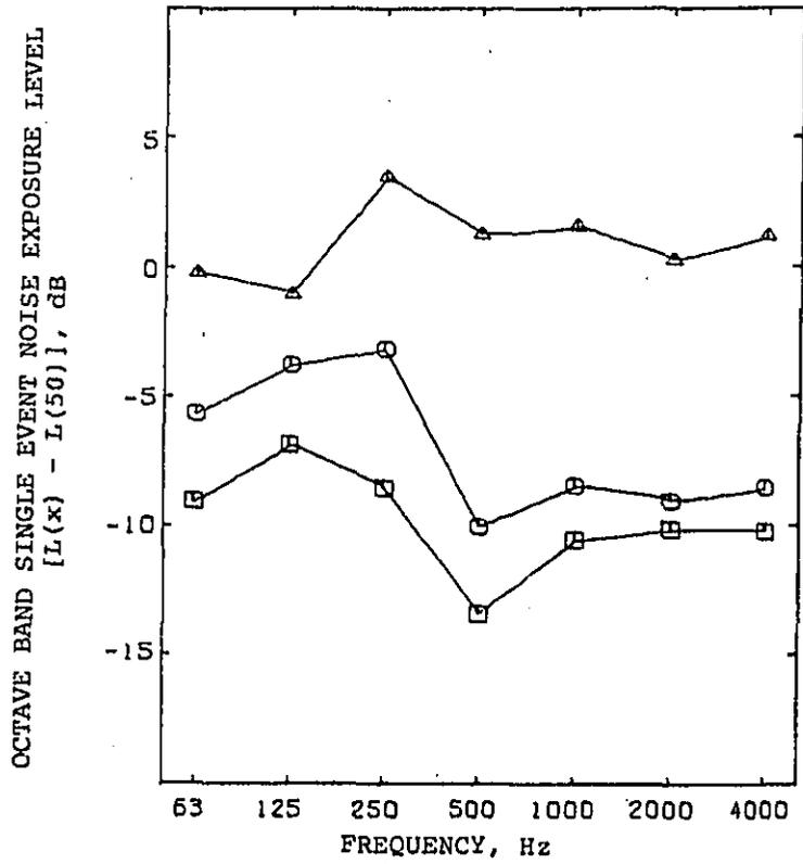
Figure 20. Octave band SENEL [L(x) - L(50)] versus frequency for east bound trains.
