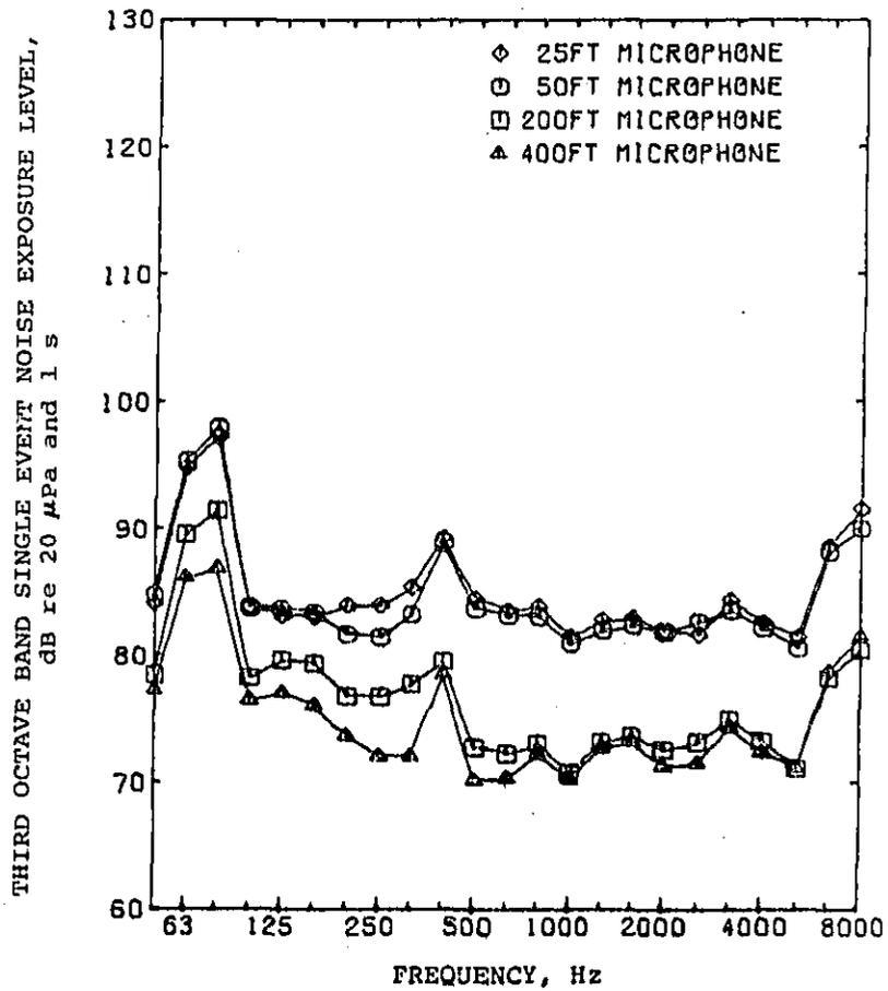
Figure 16a. Single event noise exposure level versus frequency for train no. 5983.
