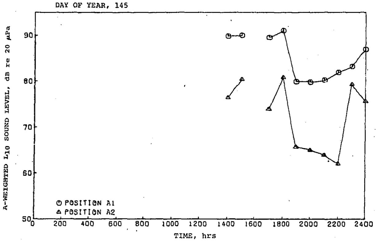
Figure 29a. A-weighted L<sub>10</sub> sound level versus time.
