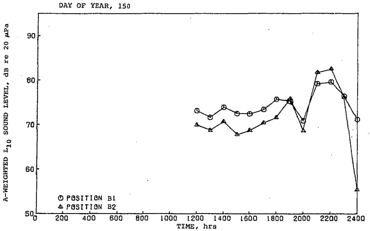
Figure 35a. A-weighted  $L_{10}$  sound level versus time.
