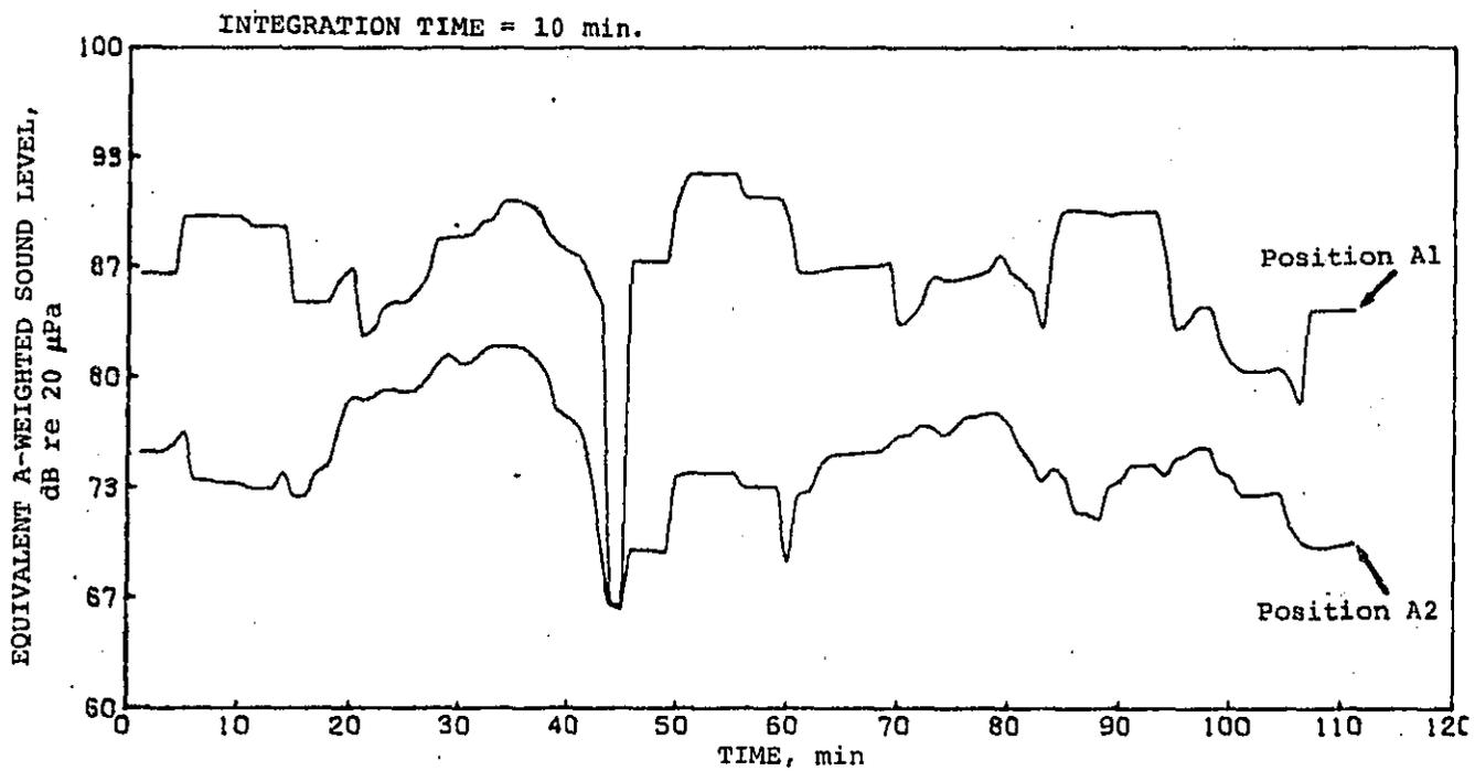
Figure 43. Equivalent A-weighted sound level versus time.
