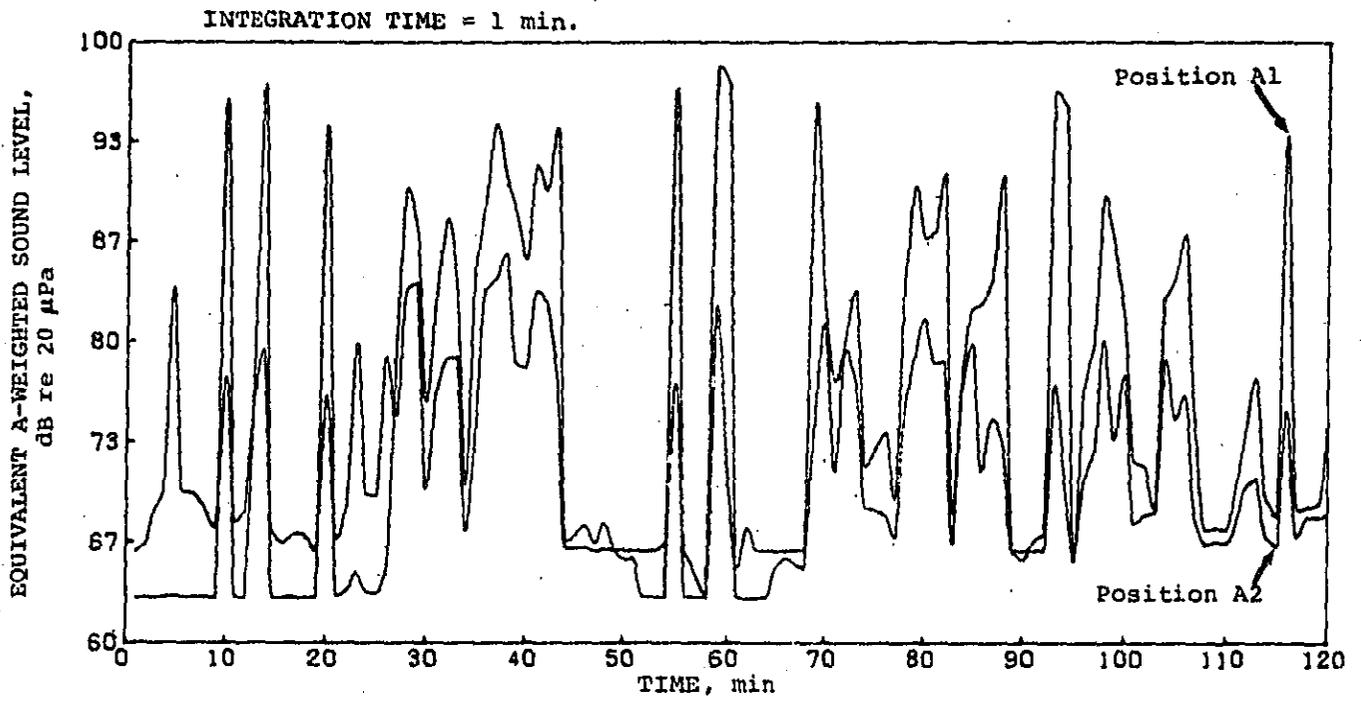
Figure 41. Equivalent A-weighted sound level versus time.
