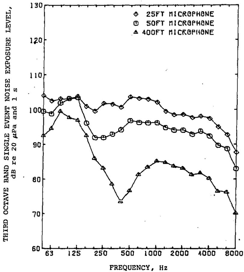
Figure 13a. Single event noise exposure level versus frequency for train no. 4031.
