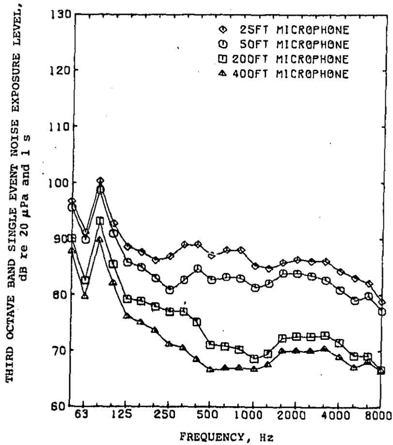
Figure 8a. Single event noise exposure level versus frequency for train no. 4054.
