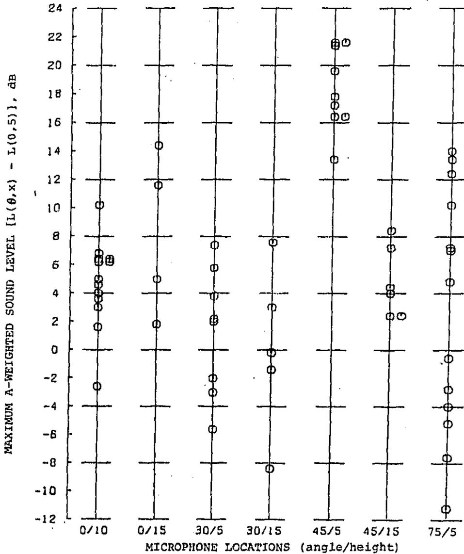
Figure 46. Maximum A-weighted sound level [L(θ,x) - L(0,5)] for various microphone locations, retarder no. 1.
