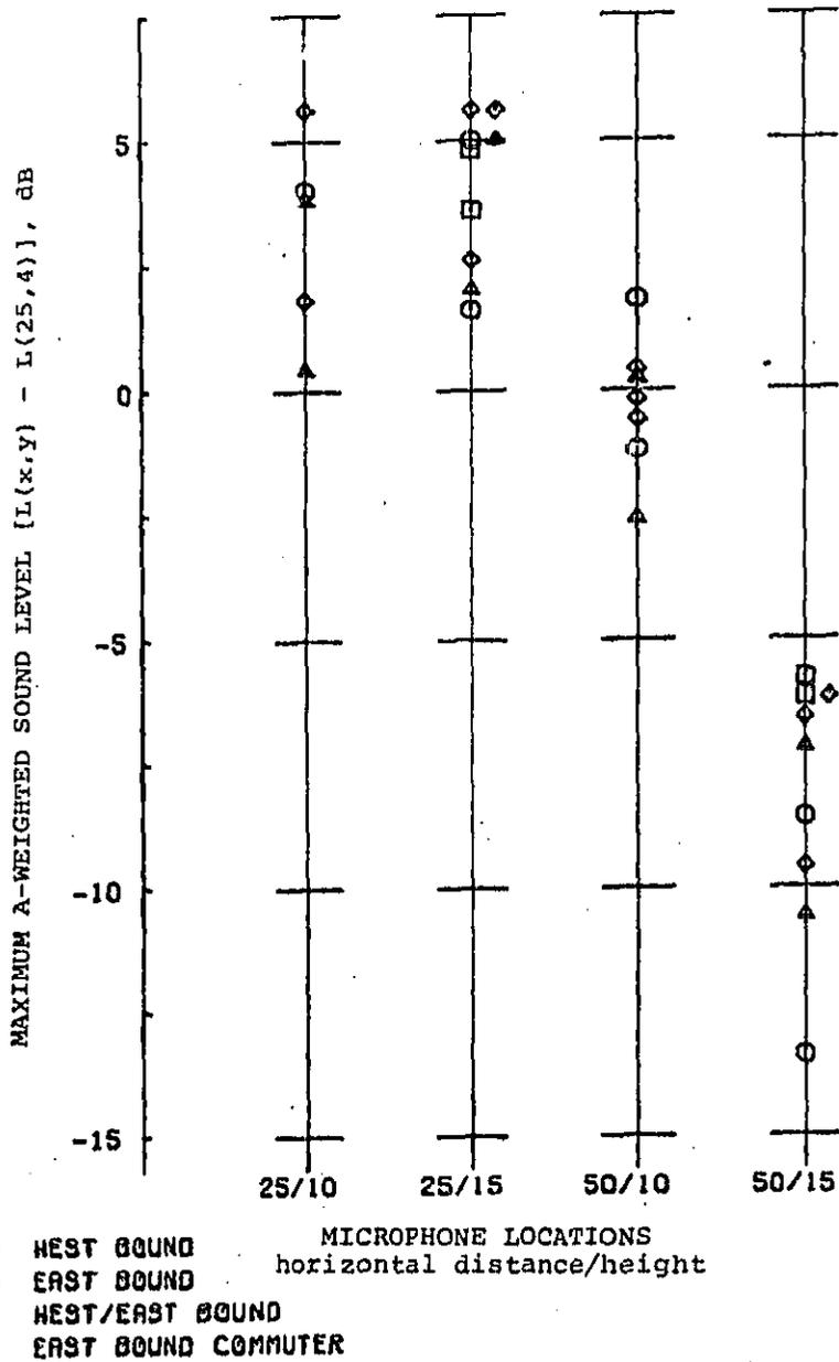
Figure 22. Maximum A-weighted sound level [L(x,y) - L(25,4)] for various microphone locations.
