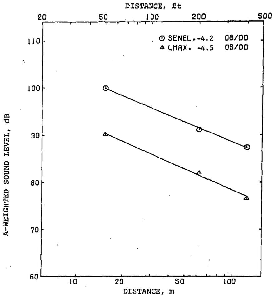
Figure 12b. Maximum A-weighted sound level (in dB re 20  $\mu$ Pa) and A-weighted SENEL (in dB re 20  $\mu$ Pa and 1 second) versus distance for train no. 6970.
