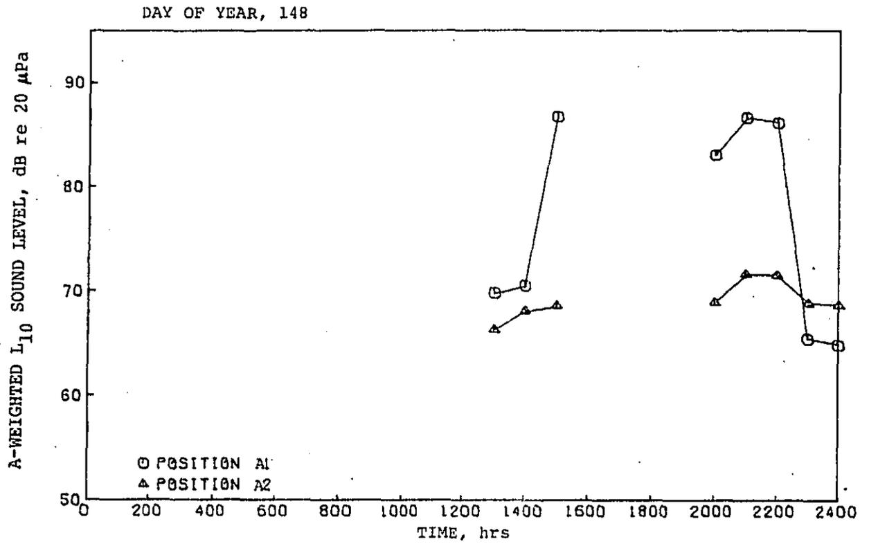
Figure 32a. A-weighted  $L_{10}$  sound level versus time.
