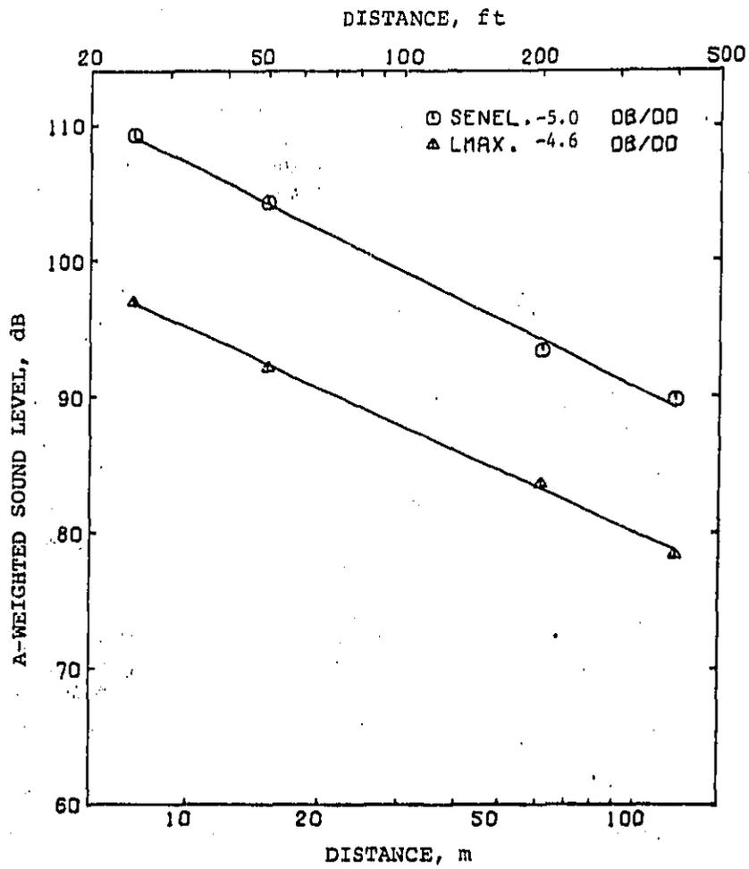
Figure 5b. Maximum A-weighted sound level (in dB re 20  $\mu$ Pa) , and A-weighted SENEL (in dB re 20  $\mu$ Pa and 1 second) versus distance for train no. 4103.
