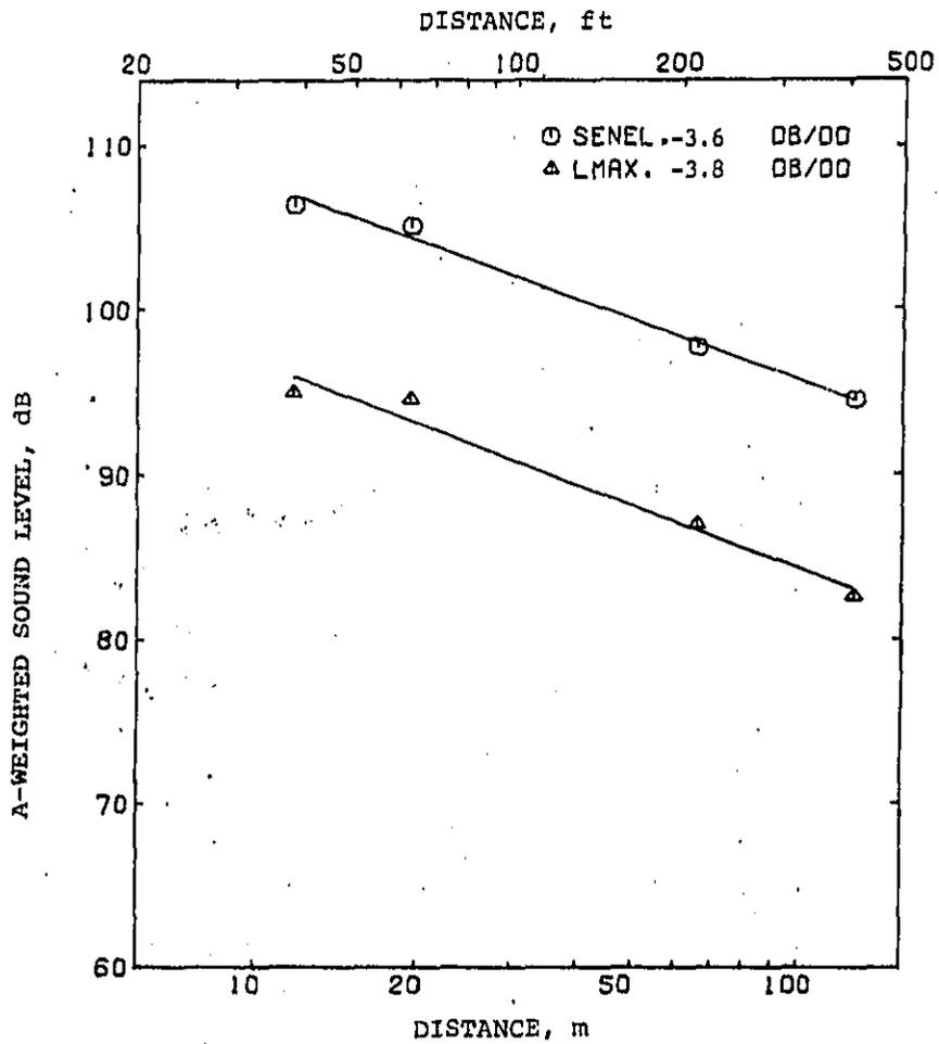
Figure 14b. Maximum A-weighted sound level (in dB re 20  $\mu$ Pa) and A-weighted SENEL (in dB re 20  $\mu$ Pa and 1 second) versus distance for train no. 3555.
