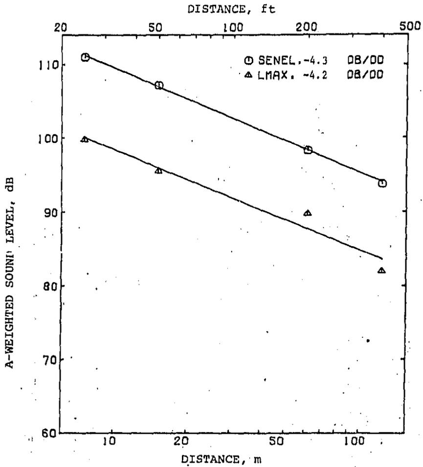
Figure 10b. Maximum A-weighted sound level (in dB re 20  $\mu$ Pa) and A-weighted SENEL (in dB re 20  $\mu$ Pa and 1 second) versus distance for train no. 4036.
