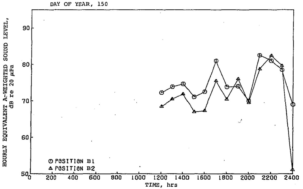
Figure 35b. Hourly equivalent A-weighted sound level versus time.
