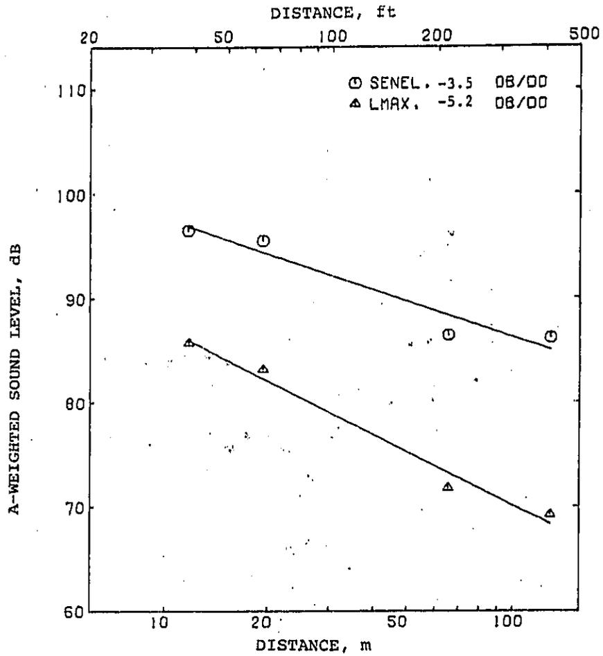
Figure 16b. Maximum A-weighted sound level (in dB re 20  $\mu$ Pa) and A-weighted SENEL (in dB re 20  $\mu$ Pa and 1 second) versus distance for train no. 5983.
