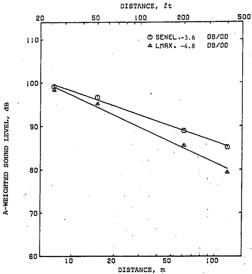
Figure 6b. Maximum A-weighted sound level (in dB re 20  $\mu$ Pa) and A-weighted SENEL (in dB re 20  $\mu$ Pa and 1 second) versus distance for train no. 6607.
