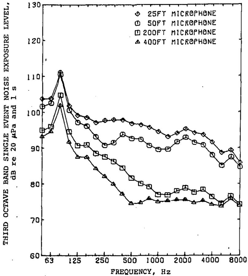
Figure 7a. Single event noise exposure level versus frequency for train no. 7411.
