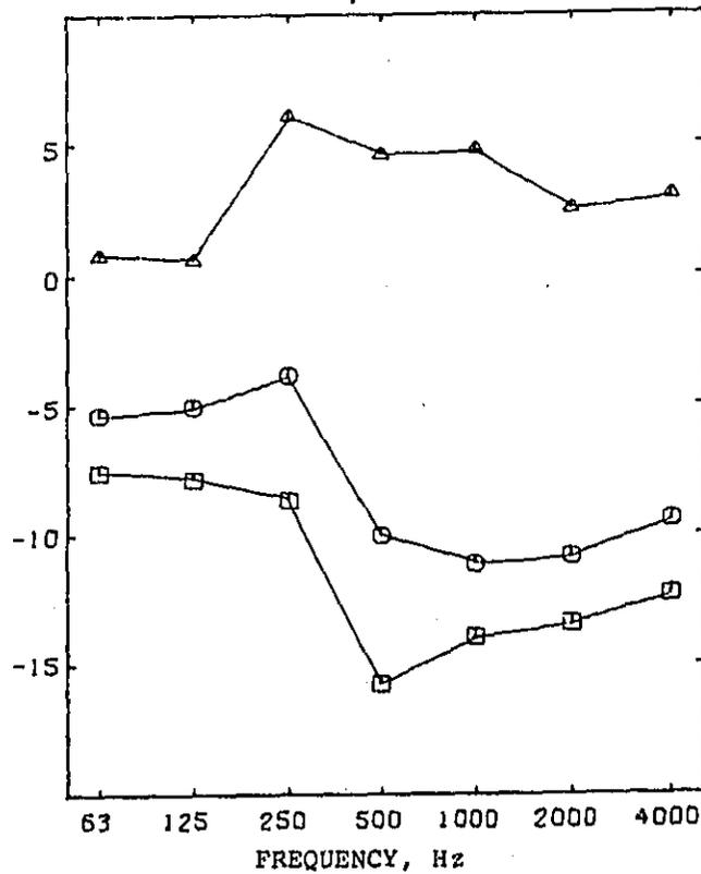
Figure 19. Octave band SENEL  $[L(x) - L(50)]$  versus frequency for west bound trains.
