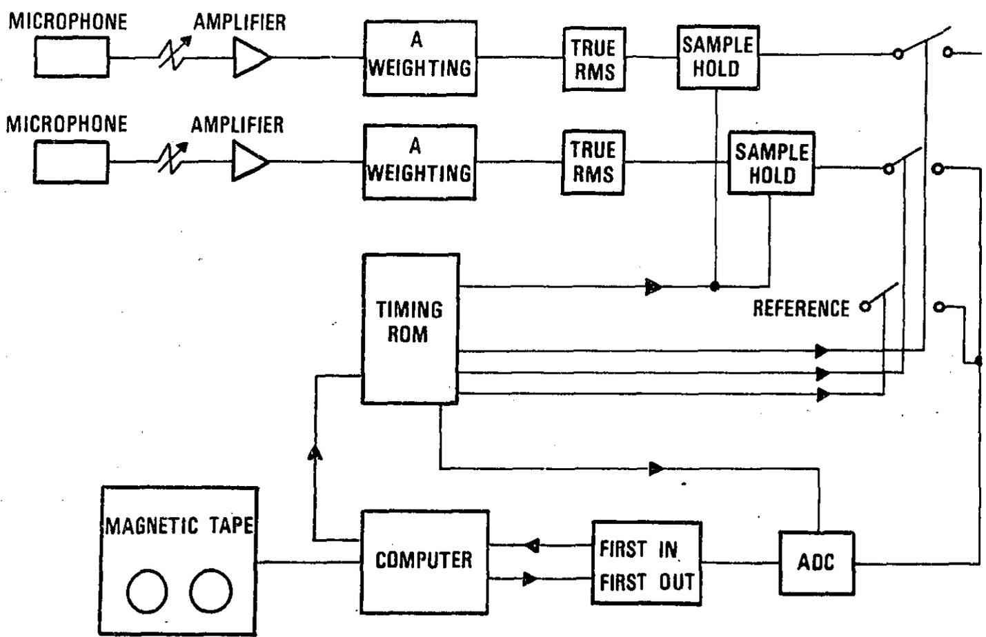
Figure C-1. Data acquisition system for yard noise.
