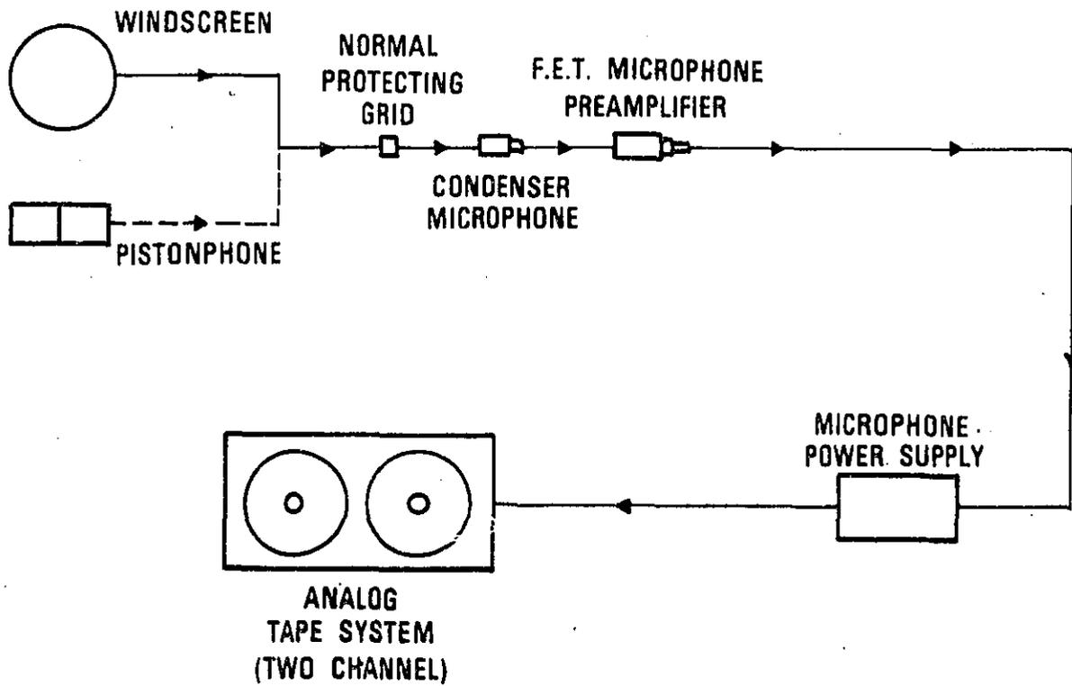
Figure D-1. Data acquisition and recording system for retarder noise.
