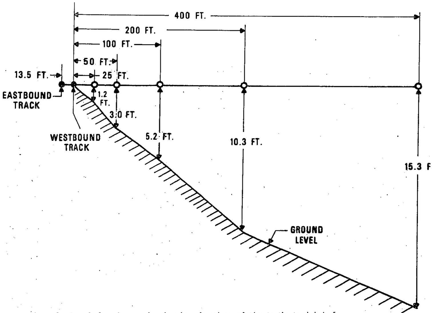
Figure 2. Ground elevations at the microphone locations relative to the track bed of the Chesapeake and Ohio main line at the Gaithersburg test site.
