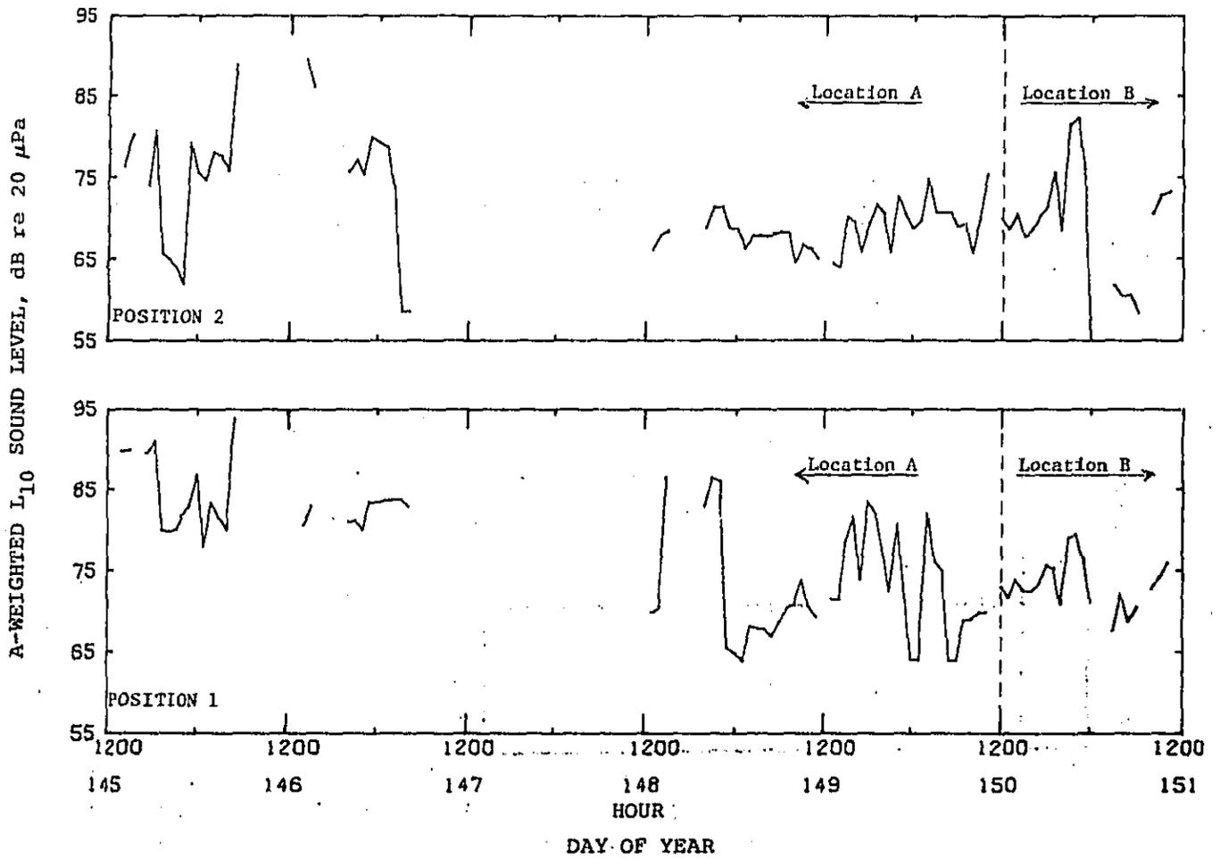
Figure 37. A-weighted L<sub>10</sub> sound level versus time.
