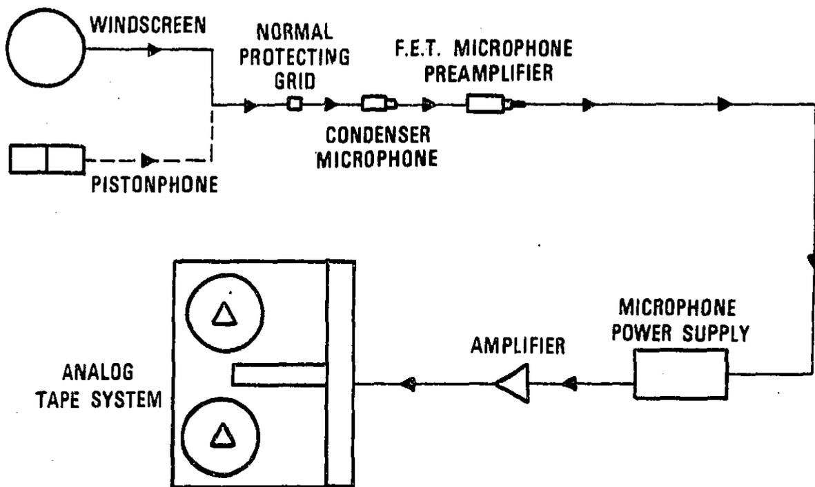
Figure A-1. Data acquisition and recording system for noise on main line.
