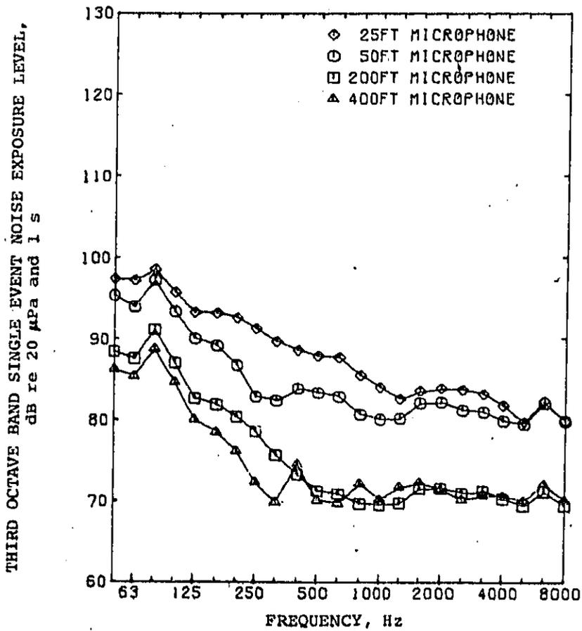
Figure 9a. Single event noise exposure level versus frequency for train no. 3823.
