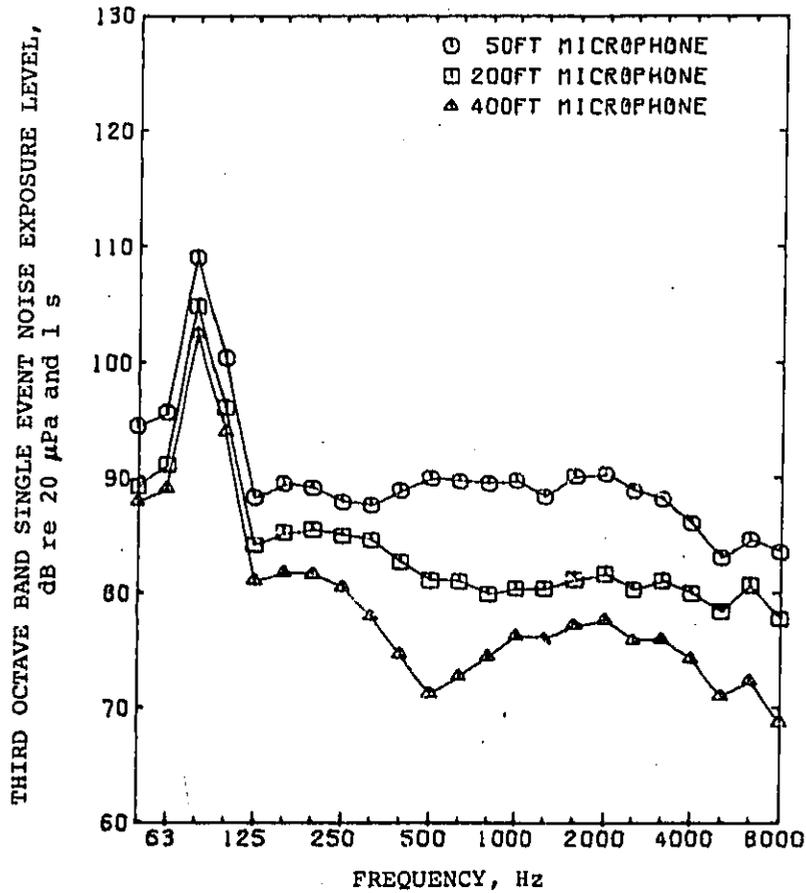
Figure 12a. Single event noise exposure level versus frequency for train no. 6970.
