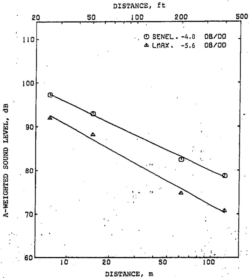
Figure 8b. Maximum A-weighted sound level (in dB re 20  $\mu$ Pa) and A-weighted SENEL (in dB re 20  $\mu$ Pa and 1 second) versus distance for train no. 4054.
